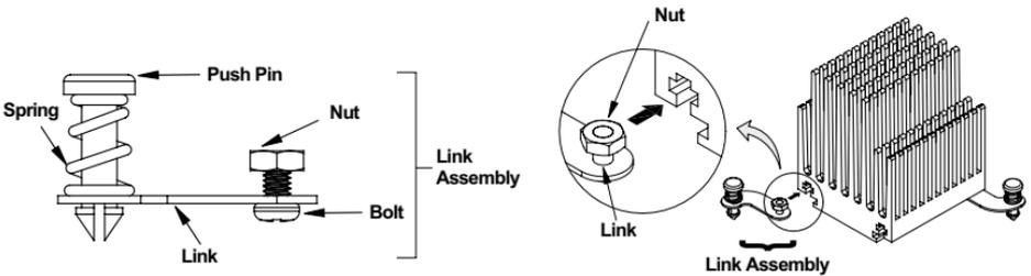
1. Insert the bolt into the bolt hole of the link and screw on the nut as shown in the diagram. Then, assemble the push pin and the spring onto the link. (The end of the spring having the smaller diameter goes with the head of the push pin.)
