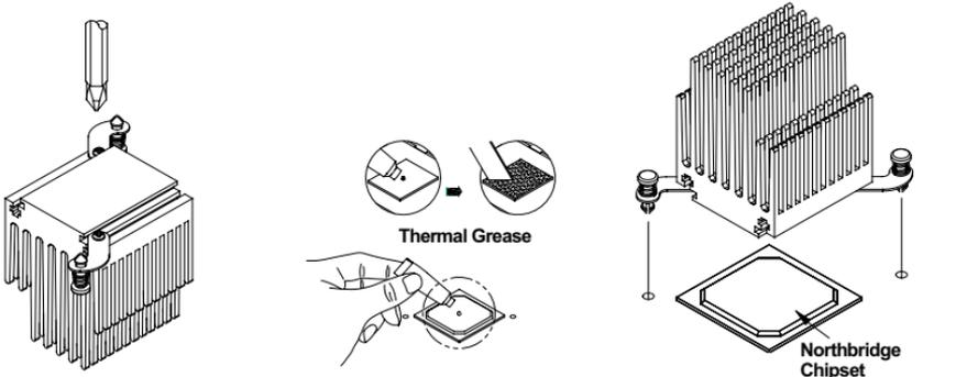
3. Align the push pins on the link assembly with the holes on the motherboard and fasten the bolts.
